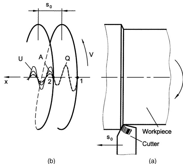
Fig. 7. External bar turning (a) and the trajectory of the cutting tool (b).
