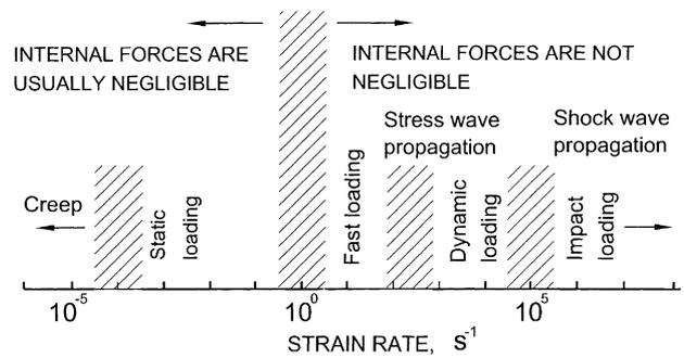
Fig. 1. Classification of various types of loading in terms of strain rate.
