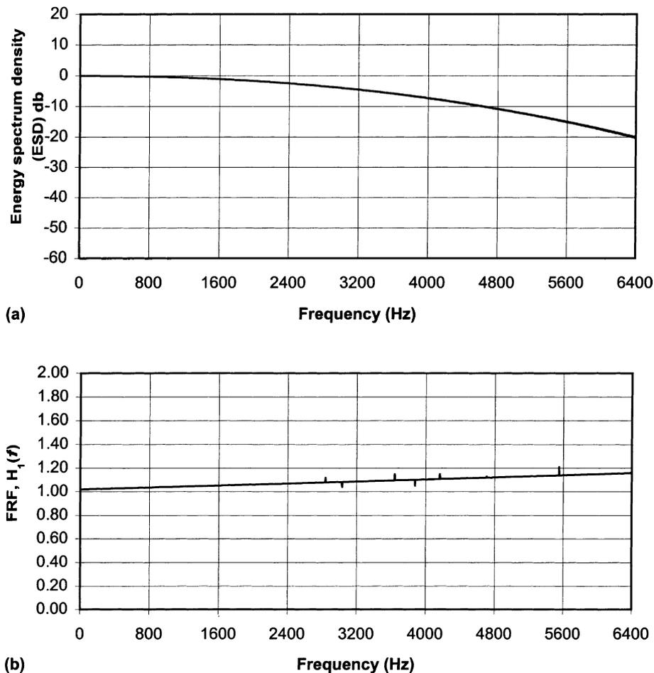
Fig. 4. Calibration of the hammer for the FRF measurements: (a) hammer response; (b) FRF values.
