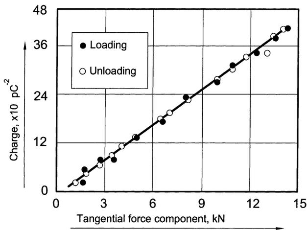
Fig. 3. Typical calibration chart (channel of the tangential force component, static calibration).
