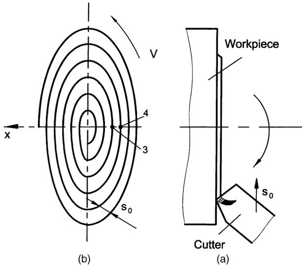
Fig. 8. Face cutting (a) and trajectory of the cutting tool (b).
