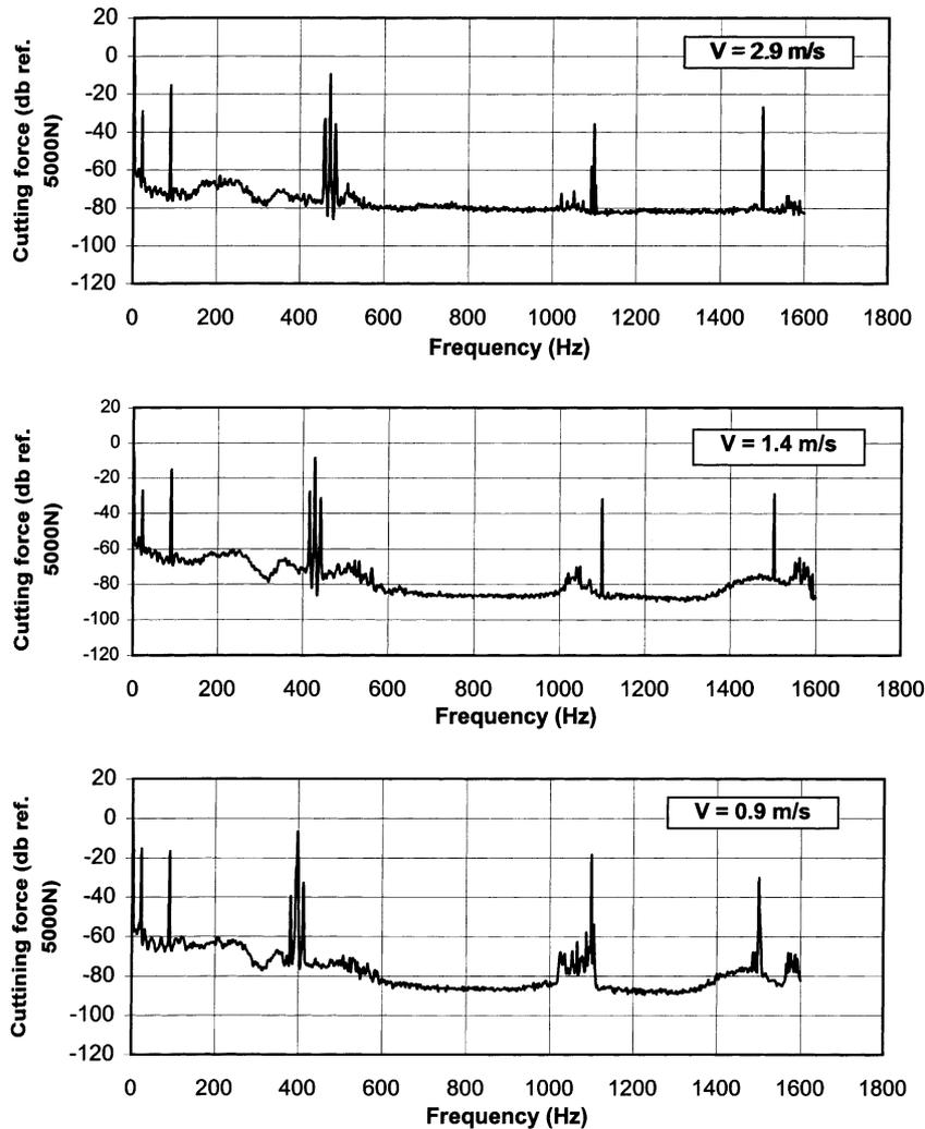
Fig. 10. Autospectras for the cutting force for different cutting speeds. Workpiece material — AISI 4140.
