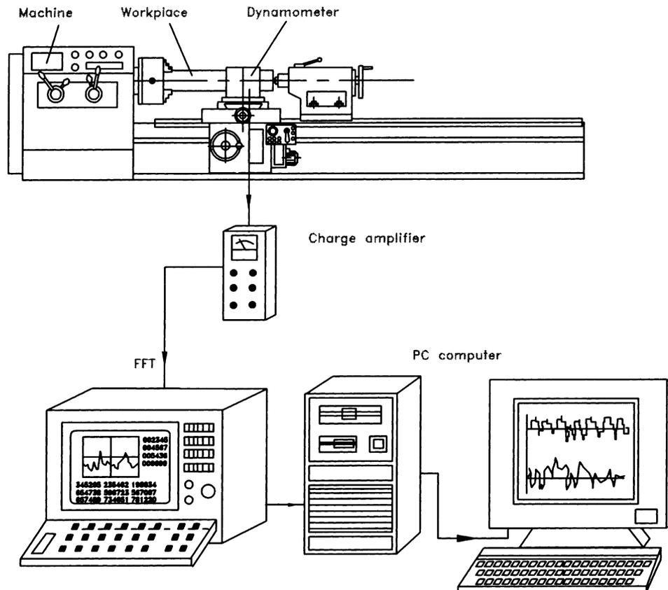
Fig. 2. Schematic diagram for measuring setup.
