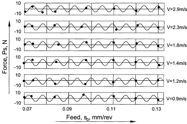
Fig. 9. Sine wave approximations of the experimental data in the coordinate system “ $P_s-s_0$ ”.
