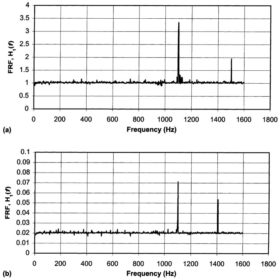
Fig. 5. FRF when the input excitation was along the direction of the power component of the cutting force: (a) direct correlation; (b) cross-correlation.
