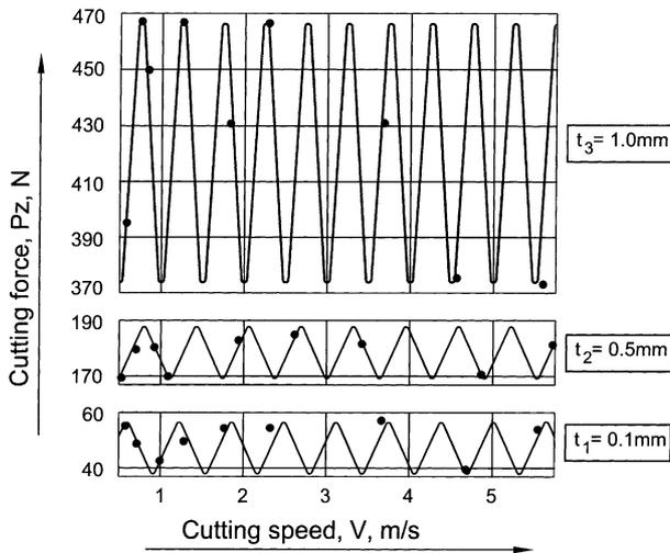
Fig. 6. Experimental results represented as sinusoidal periodic data in the coordinate system “ $V-P_z$ ”: (a)  $t_1 = 0.1$  mm; (b)  $t_2 = 0.5$  mm; (c)  $t_3 = 1.0$  mm.
